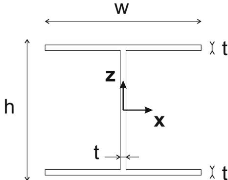
Figure 2: Cross-section of the I shaped beam.
