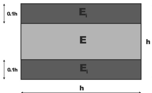
Figure 3: Damage distribution above the cross-section of the orthotropic beam
