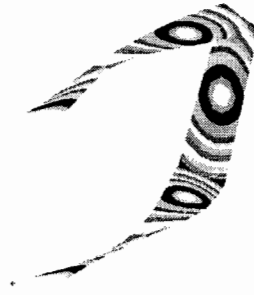
Figure 9: Natural mode of a joined wing. Shell model solution. f = 47.118 [Hz] [42]
