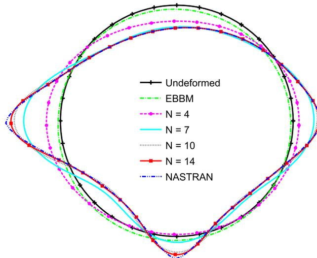
Fig. 12. Static response of the mid-span circular cross-section,  $t=0$  s.
