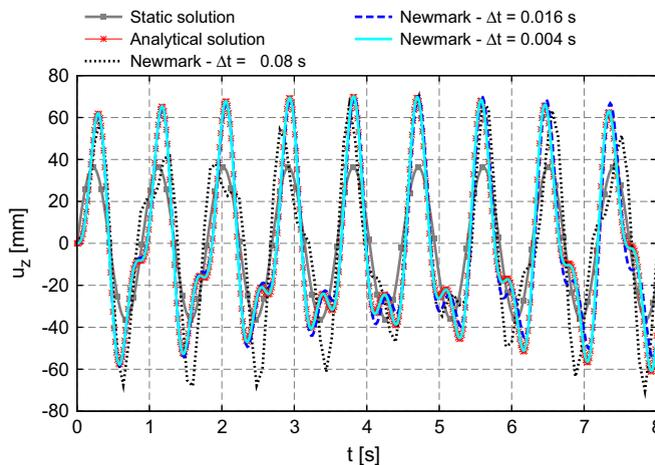
Fig. 2. Effect of the time step  $\Delta t$  on the transverse displacement at the mid-span section. Square cross-section case. Sinusoidal load. EBBM.
