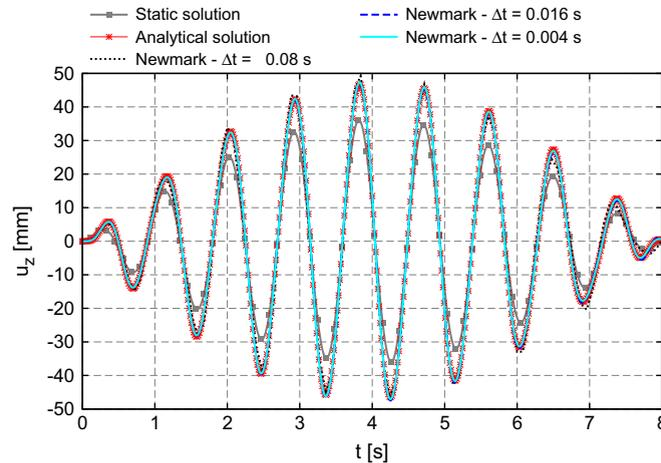
Fig. 3. Effect of the time step  $\Delta t$  on the transverse displacement at the mid-span section. Square cross-section case. Sinusoidal traveling load. EBBM.
