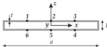
Fig. 5. Thin-walled rectangular cross-section.
