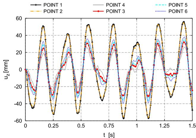
Fig. 8. Dynamic response of different points on the loaded cross-section. Thin-walled rectangular cross-section case,  $\Delta t = 7.5 \times 10^{-4}$  s,  $N=10$ .
