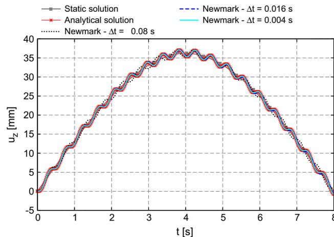
Fig. 4. Effect of the time step  $\Delta t$  on the transverse displacement at the mid-span section. Square cross-section case. Constant traveling load. EBBM.
