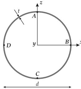
**Fig. 11.** Thin-walled circular cross-section.
