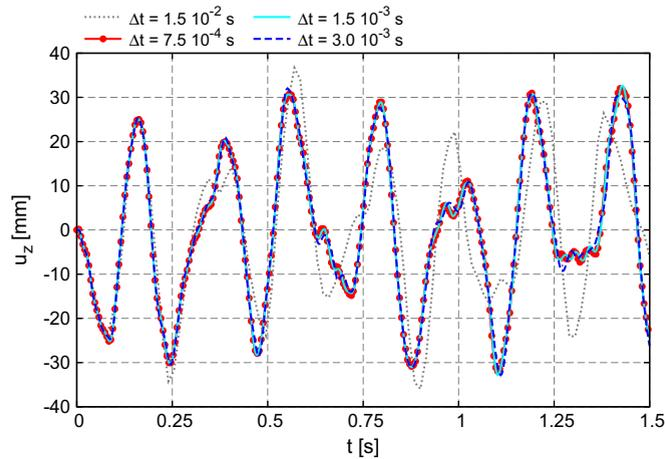
Fig. 7. Effect of the time step  $\Delta t$  on the transverse displacement of point 3. Thin-walled rectangular cross-section case,  $N=10$ .
