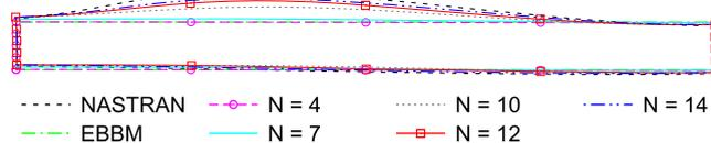
Fig. 6. Static deformation of the loaded thin-walled rectangular cross-section.
