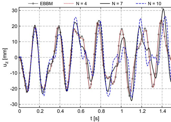
Fig. 10. Time-dependent transverse displacement of point 4 for different theories. Thin-walled rectangular cross-section case,  $\Delta t = 7.5 \times 10^{-4}$  s.
