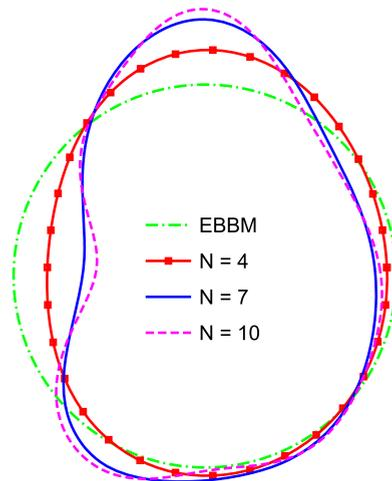
Fig. 14. Deformation of the mid-span circular cross-section for different beam models,  $t=0.025$  s.
