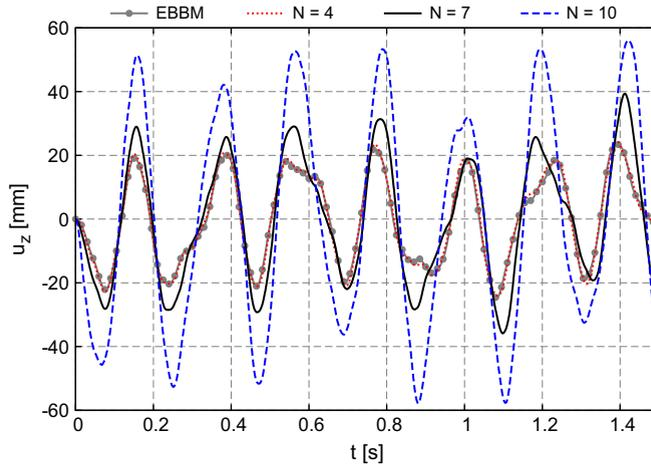
Fig. 9. Time-dependent transverse displacement of point 1 for different theories. Thin-walled rectangular cross-section case,  $\Delta t = 7.5 \times 10^{-4}$  s.
