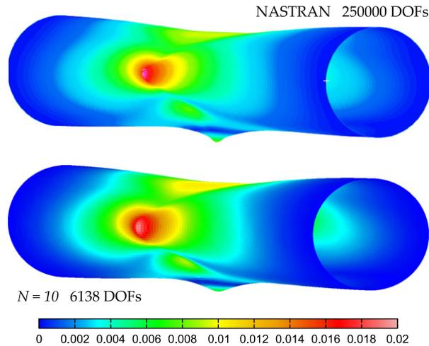
Fig. 13. Static three-dimensional resultant displacement of the thin-walled cylinder,  $t=0$  s.
