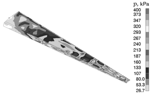
Fig. 7. Effect of an explosion of an HE equivalent to 16-kg TNT mass on the wing box.
