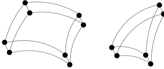
**Figure 16.** Rectangular and triangular FE degenerated elements
