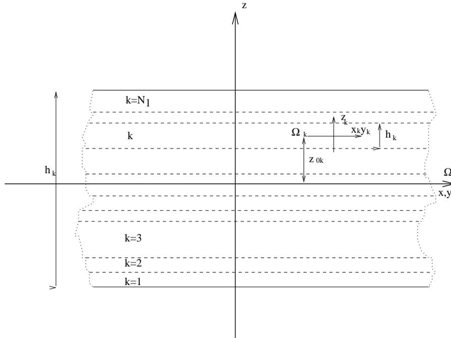
**Figure 4.** Notations for a multilayered plate
