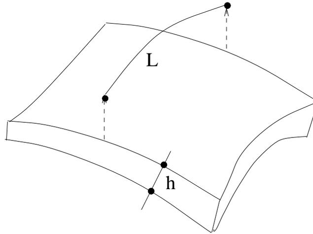
**Figure 3.** Geometrical parameters in a two-dimensional structure  $h/L \ll 1$
