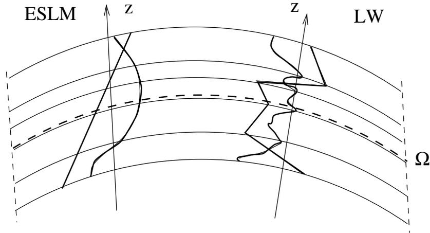
**Figure 7.** Linear and Higher  $z$ -expansion in a layered shell. Comparison between LWM and ESLM assumptions
