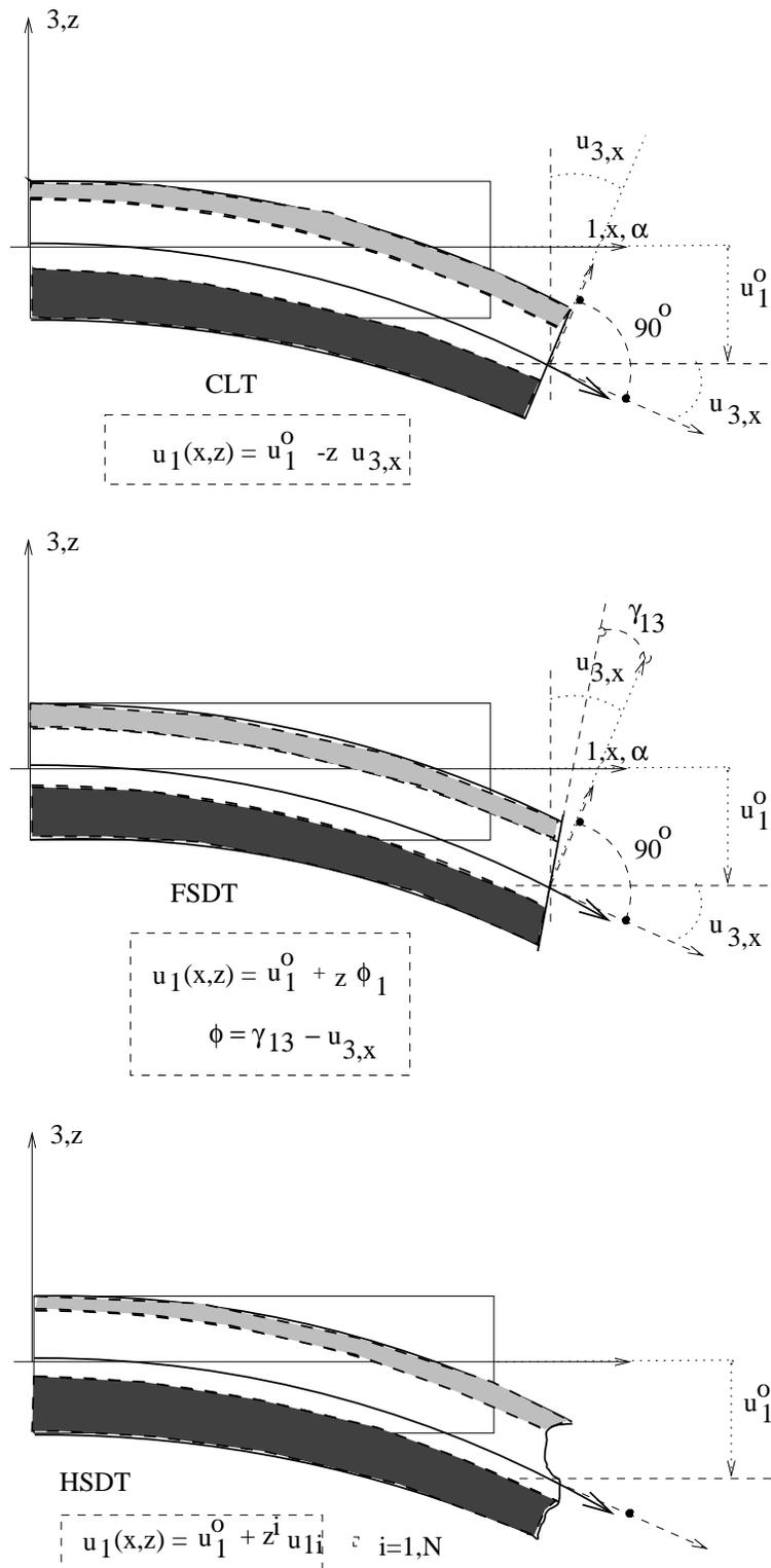
Figure 10. CLT, FSDT and HSDT assumptions in one-dimensional cases
