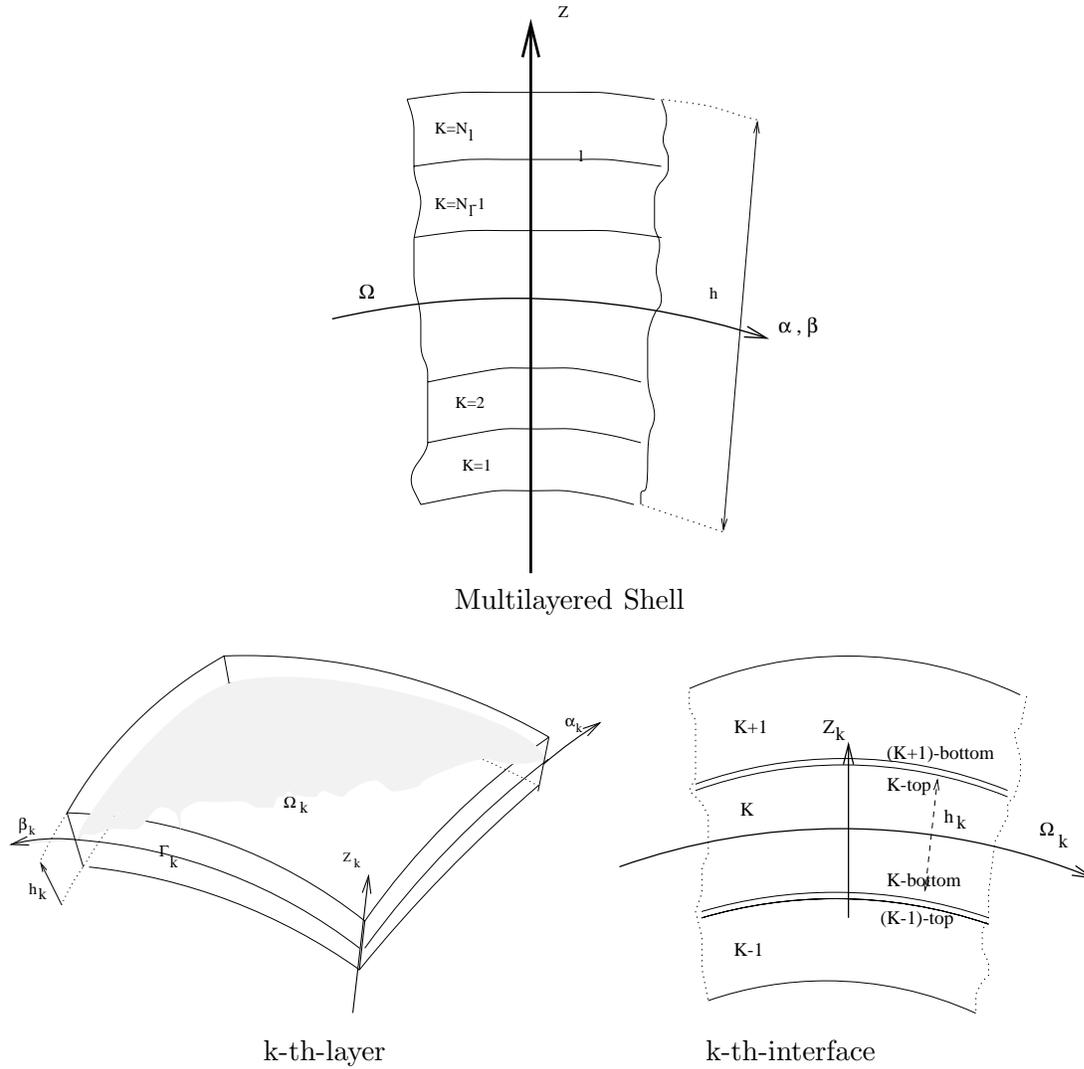
Figure 5. Geometry and notations used for multilayered shells
