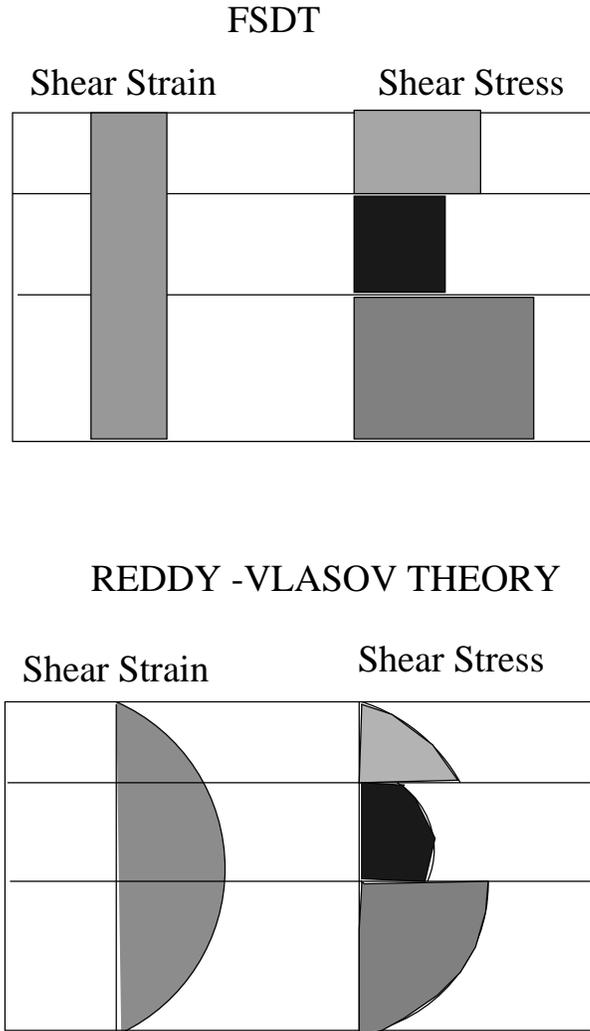
**Figure 11.** Shear strains and stresses for FSDT and Reddy–Vlasov theory
