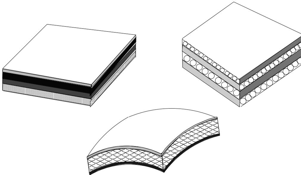
**Figure 1.** Examples of multilayer structures. Plates (upper part) made of layers of different materials (left) and by unidirectional fibers (right) and sandwich shell (upper part)
