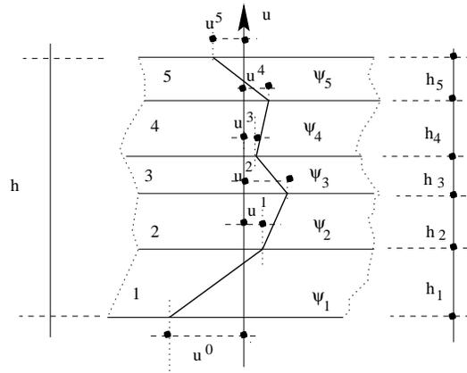
**Figure 12.** Geometry and notations employed to introduce zig-zag theories
