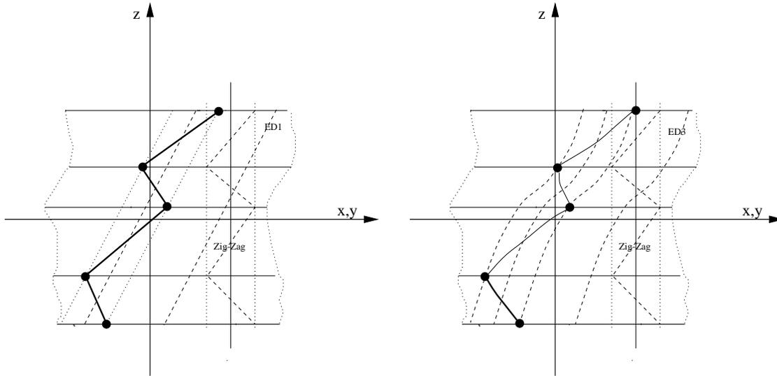
**Figure 14.** Geometrical meaning of Murakami's zig-zag function. Linear case and higher order cases
