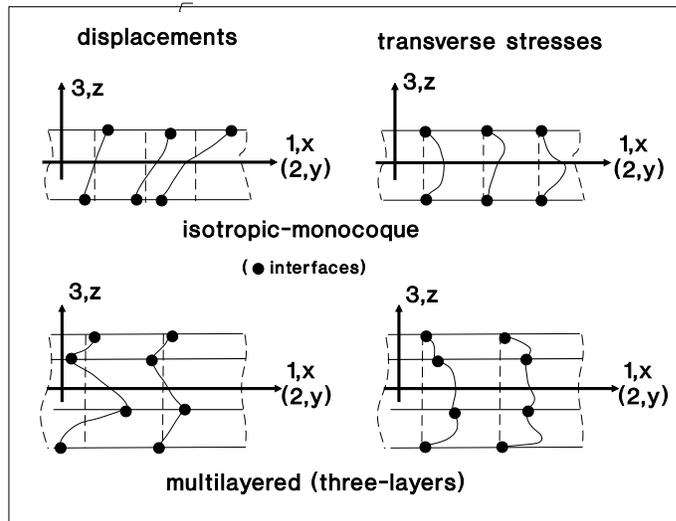
Figure 8.  $C_z^0$ -Requirements. Comparison of transverse stress field between a one-layer structure and a three-layer structures
