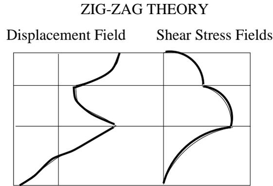
**Figure 13.** Displacement and transverse stress field for a Zig-Zag type theory
