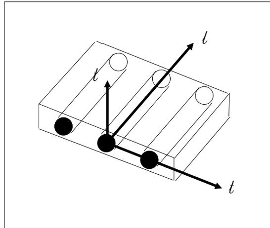
**Figure 2.** Unidirectional lamina
