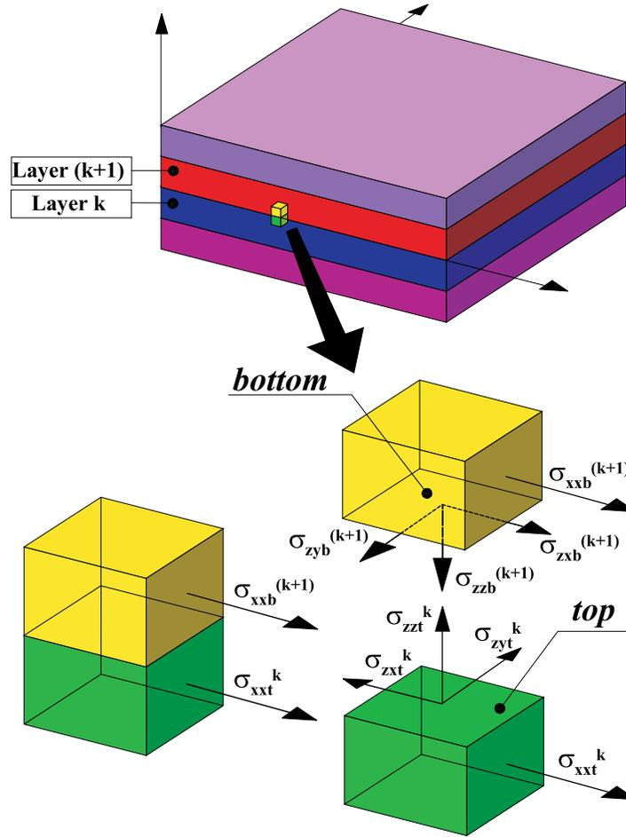
**Figure 9.** Details and notations of stresses at the interface
