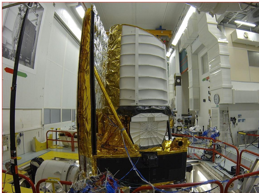
Figure 1 Euclid Spacecraft on the shaker at Thales-Alenia Space Test Facilities in Cannes (F)
